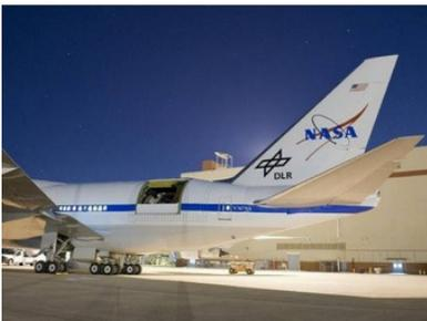
Outside view of the back end of the plane, with a sliding door, to point telescope to the star birthing area of the universe for astronomical research
